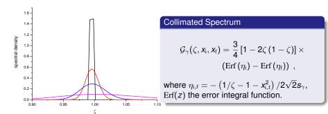
For pin-hole collimation energy spread of gammas is the doubled spread of electrons (plus spread of the laser photons energy)
