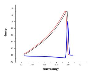
Substraction of the images produced by spectra with slightly different energies of electrons resembles spectral width  $\geq$  2× beam energy spread
