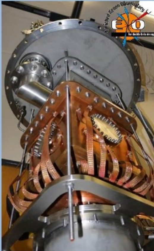
Photograph of the inner chamber of the cryostat along with the LN 2 tank showed below
