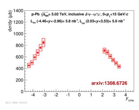
y>0 (red) is the p-going direction. Probes small x in the Pb nucleus ( $\sim 10^{-5}$ ) y<0 (blue) is the Pb-going direction. Probes large x in the Pb nucleus ( $\sim 10^{-2}$ )
