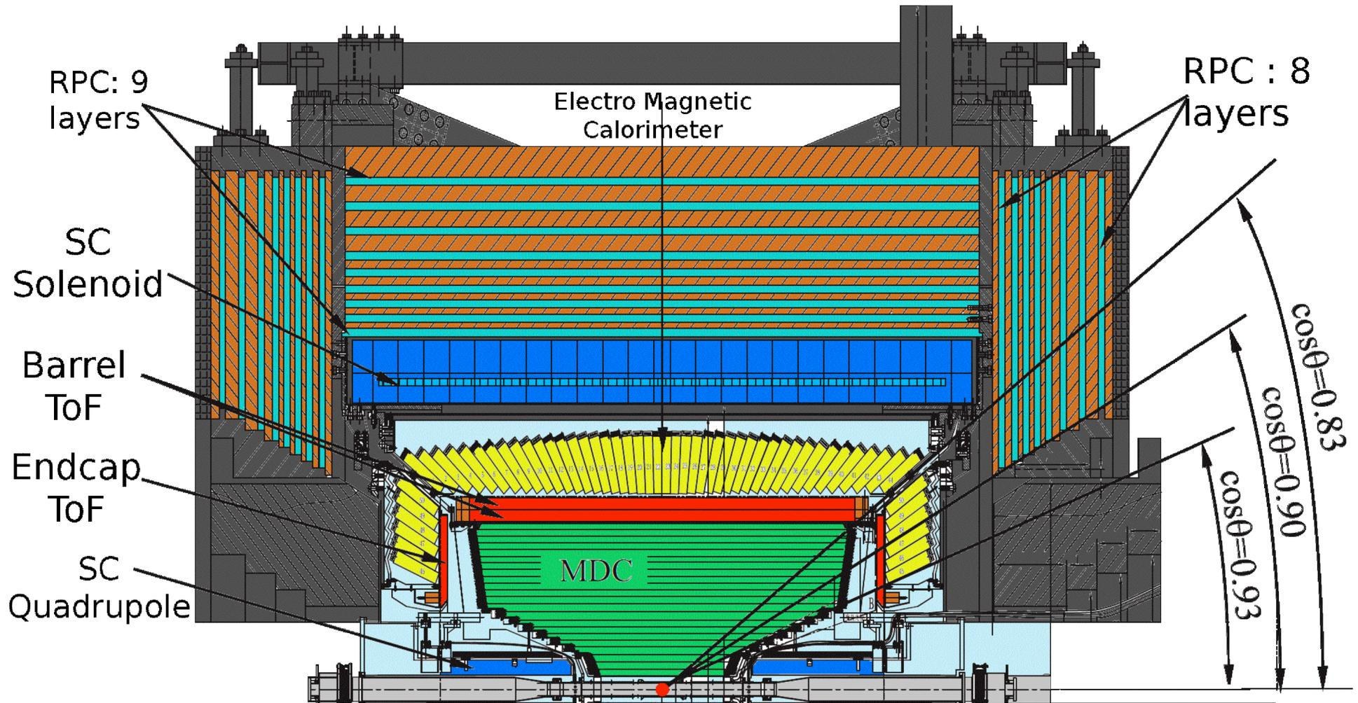
**Wire tracker** (no Si); **TOF** + **dE/dx** for PID; **CsI Ecal**; **RPC muon**
