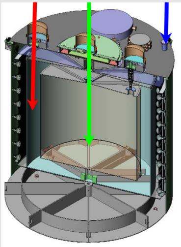
Load cells measure 20 ton target mass to 3 kg (0.015%)
