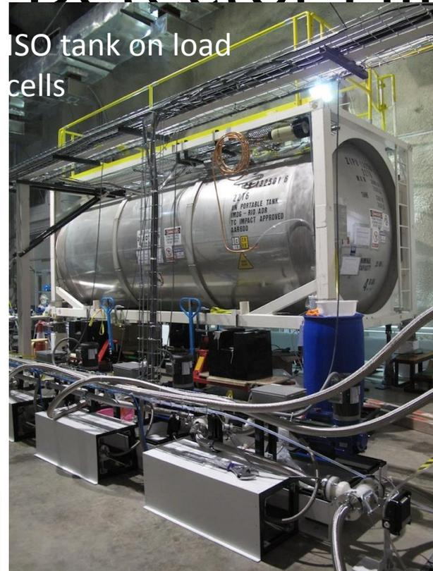
ISO tank on load cells
