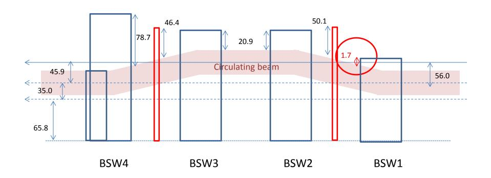
35 mm from KSW for horizontal painting 45.9 mm from BSW chicane bump
