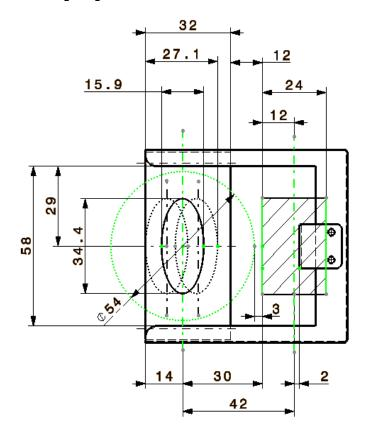
Estimated beam size on the foil for zero dispersion (left) and matched (-1.4 m) dispersion (right) at injection point. PSB beam envelope (Ø54mm) during injection is also shown. (L4-T-EP-0005, EDMS 1108941)
