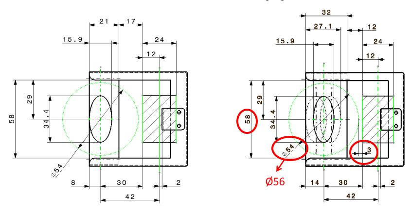
Estimated beam size on the foil for zero dispersion (left) and matched (-1.4 m) dispersion (right) at injection point. PSB beam envelope (Ø56mm) during injection is also shown. (L4-T-EP-0005, EDMS 1108941)
