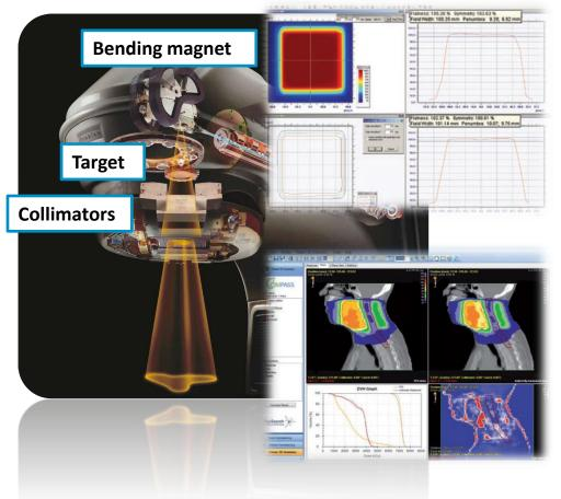
Before starting daily patient treatments, it is important to perform <u>QA measurements</u> in order to check critical LINAC parameters such as penumbra, symmetry, flatness and field size
