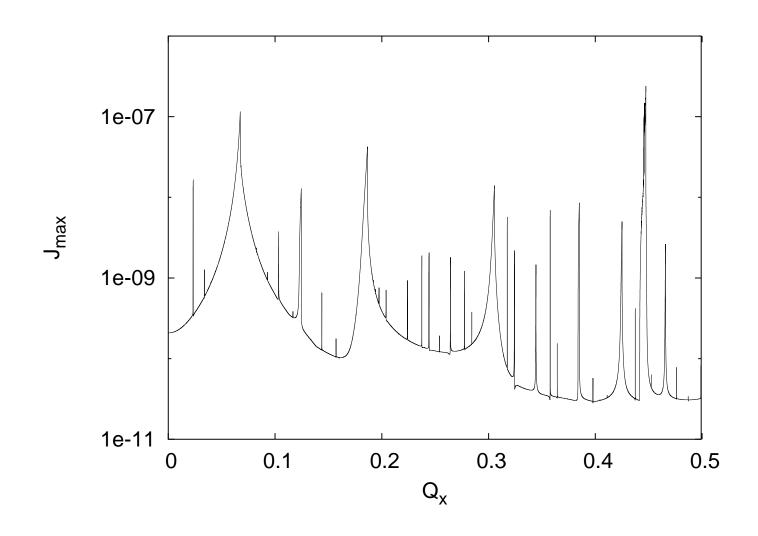
eRHIC emittance growth at the polarized proton working point (.695/.685), for the same crab cavity harmonics
