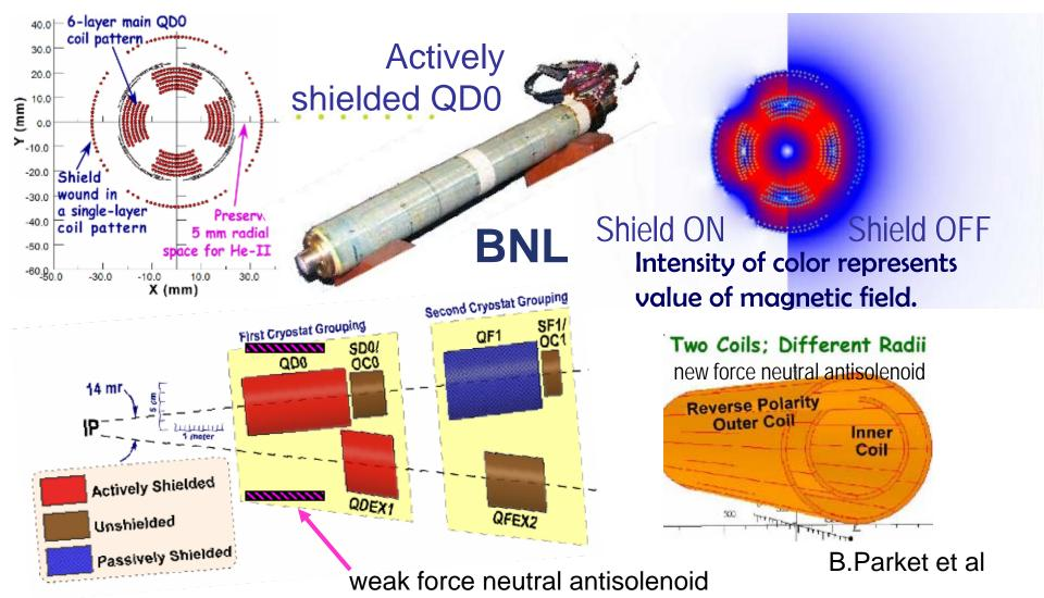
Final doublet includes self shielding quads, sextupoles for chromatic corrections, octupoles for higher order aberrations, weak antisolenoid to correct coupling, dipole and skew corrections for orbit tuning, etc.
