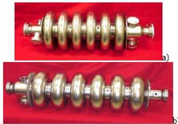
Figure 1: SNS  $\beta=0.61$  (a) and  $\beta=0.81$  (b) cavities.
