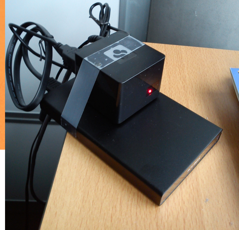
Cubox ARM computer ARM Cortex A9, 800MHz eSata connector and RHEL clone running “RedSleeve”
