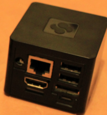
Cubox ARM computer ARM Cortex A9, 800MHz eSata connector and RHEL clone running “RedSleeve”
