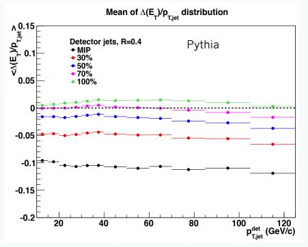
$$E_{\text{cluster}}^{\text{corr}} = E_{\text{cluster}}^{\text{raw}} - f \sum P_{\text{track}}^{\text{matched}}, \quad E_{\text{cluster}}^{\text{corr}} \ge 0$$
