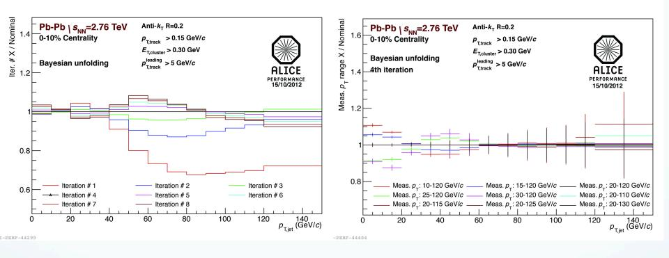
Left plot shows the effect of regularization using Bayesian unfolding Right plot show unfolding uncertainty due to measured  $p_{\text{T,iet}}$  range
