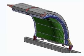
EMCal is a Pb-scintillator sampling calorimeter which covers:
