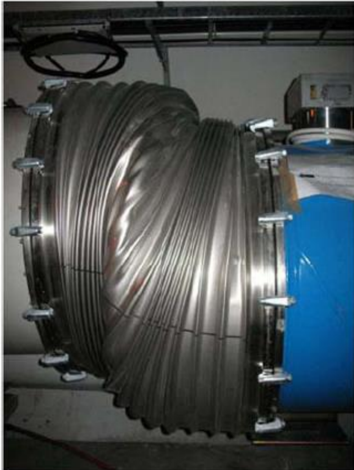
Figure 14: Damage to interconnection QQBI.27R3 by excess compression
