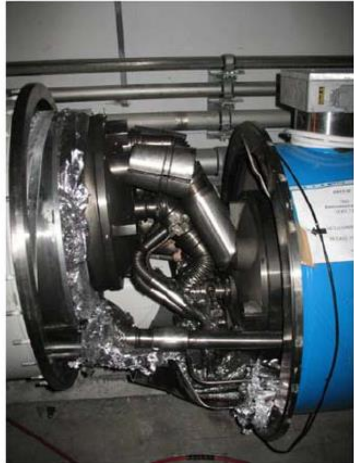
Figure 14: Damage to interconnection QQBI.27R3 by excess compression
