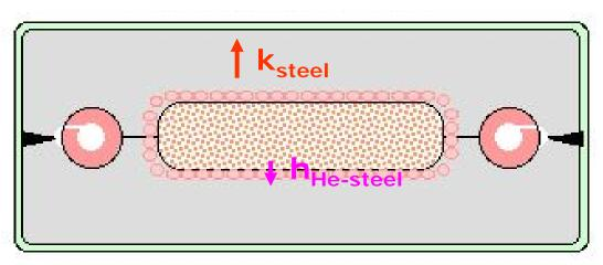
k<sub>steel</sub> ... heat conductivity (known and tabulated as function of T for different kinds of steel).
