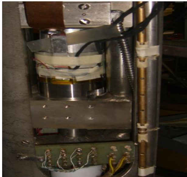
Compressive I_c test setup (LN2 testing)
