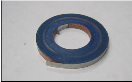
Pancake coil fabricated from 12mm wide SP 2G HTS
