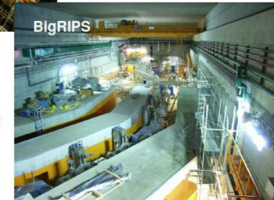
World's Largest Acceptance 9 Tm Superconducting RI beam Separator
