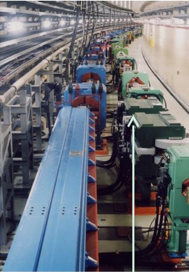
New beam pipe & bellows
