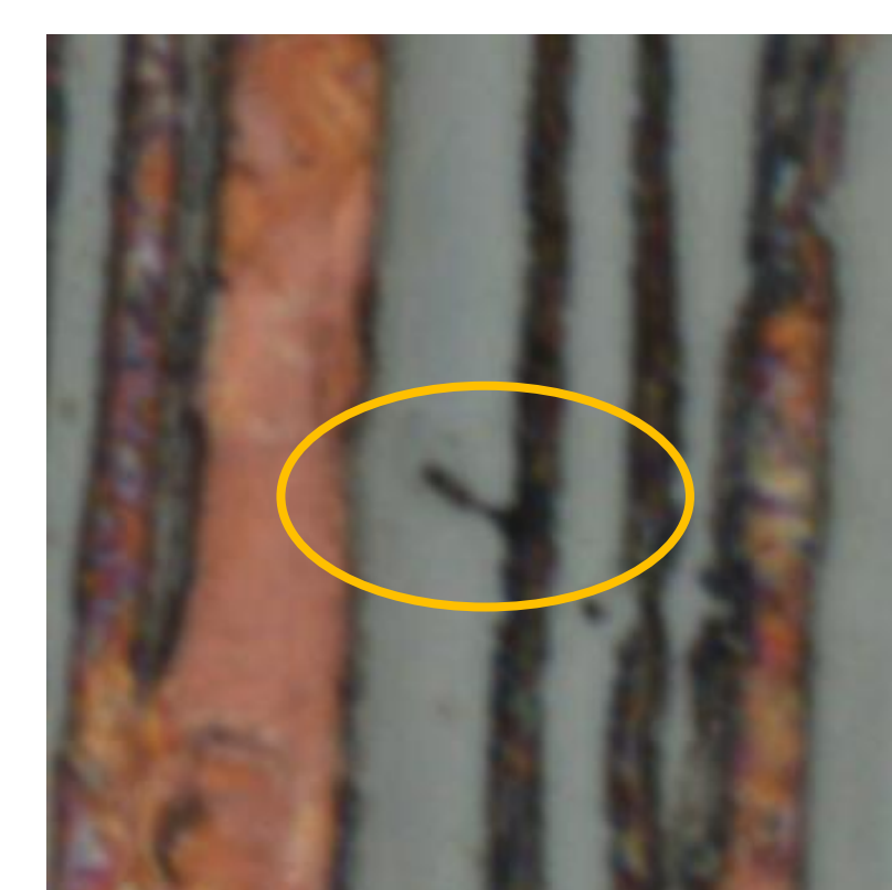
Cracks extends over a half of filament width
