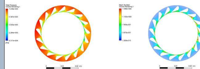
Figure 4. Contours of total pressure and mach number in the nozzle
