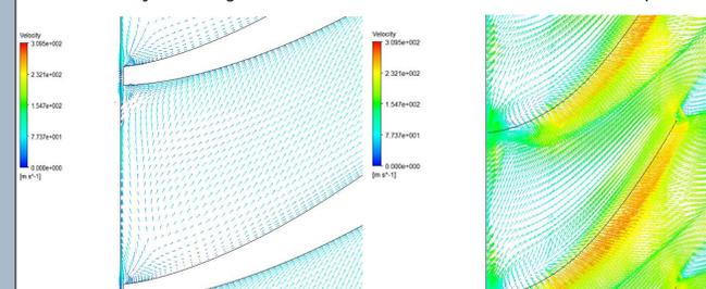
Figure 5. Velocity vector plot in the blade to blade view (a) nearer to the hub (b) nearer to the tip
