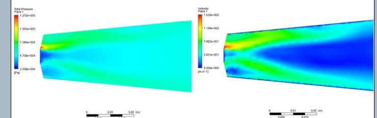
Figure 5. Contours of total pressure and velocity in the diffuser
