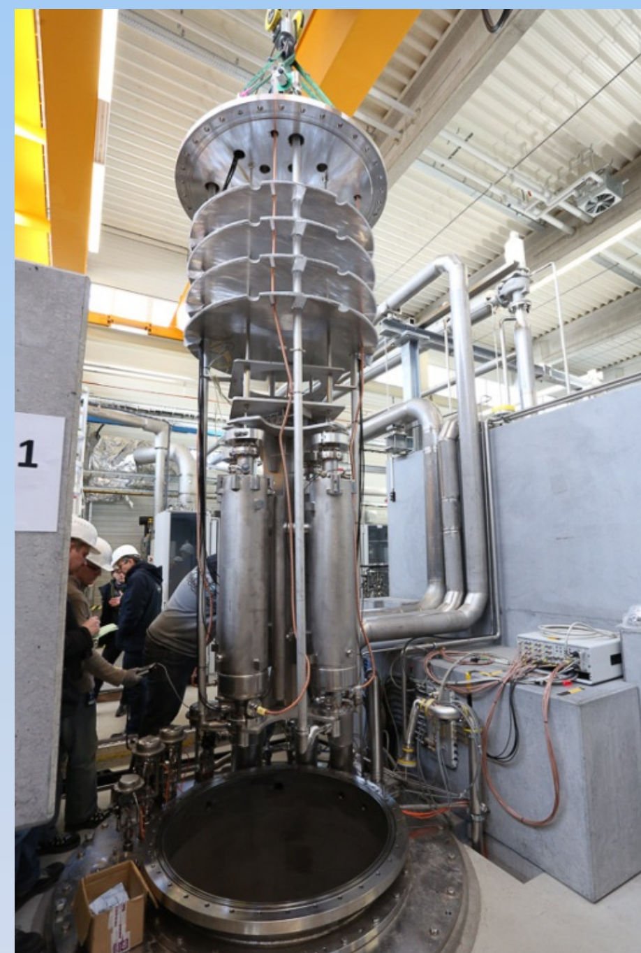
A vertical Insert for the Cavity cold test at the AMTF
