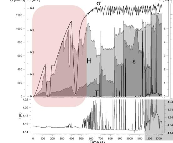
( $\sigma$ ) stress; ( $\epsilon$ ) unit strain for 10 mm region in the middle of the sample;
