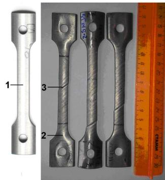
Samples were made from tubes «as received» as well as after complete simulation of the production cycle in manufacturing of conductors for ITER magnet system,
