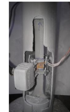
Stress was measured by a sensor located on the machine frame.
