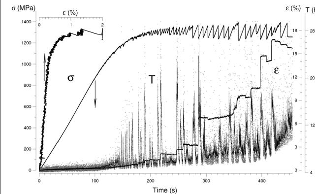
( $\sigma$ ) stress, arrows point to horizontal axes corresponding to curves;
