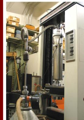
To create low temperatures the load-carrying cryostat of submersible type with allowable force to 40 kN was used.
