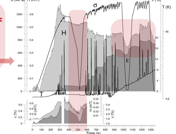
( $\sigma$ ) stress; ( $\epsilon$ ) unit strain for 10 mm region near the weld;
