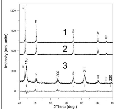
Typical X-ray diffraction patterns ( $T=300\text{ K}$ ,  $\text{CuK}\alpha$ ) for samples before (1) and after (2, 3) tensile tests below 7 K. The regions 1, 2 and 3 see in previous Figure.
