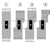
Schemes of deformation for the region under test corresponding to points 1, 2, 3 and 4 in the  $\epsilon$  curve. Black rectangle is region where strain is measured, and white circle marked by T is area where temperature is measured. Arrows show stress (in schemes 1 and 3, grey lines correspond to subsequent slips) and an elastic force when stress drops as slip happens (in schemes 2 and 4).
