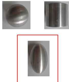
There were obvious difference between installing or no installing adjustment setup. It showed maximum 20.2% electric power increasing when appropriate ellipsoid was installed with about 10.3% system efficiency improvement. Increase of length of major axial could improve the performance.
