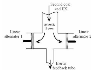
The space between pistons are seen as acoustic tube. Its equivalent length can affect the acoustic power transmitting into the alternator. Decreasing the length will decrease the input impedance of branches, then improve the performance. Placing filling in the connecting port can decrease the length.
