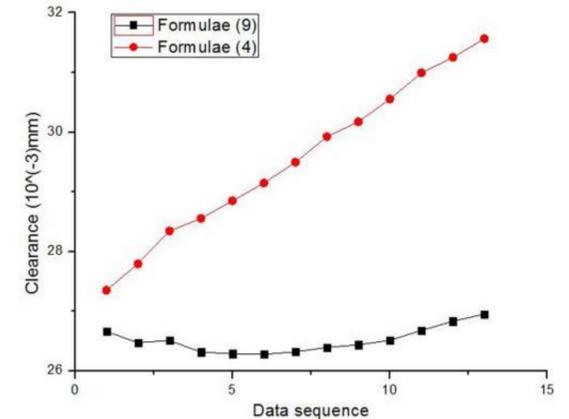
Formula (4) based on volume leakage  $\delta = \left( \frac{12\mu L Q}{(p_1 - p_2)\pi D} \right)^{\frac{1}{3}}$
