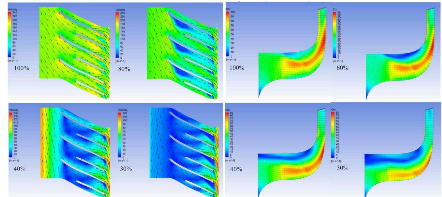
Velocity vectors at 80% span under the different reduced mass flow conditions
