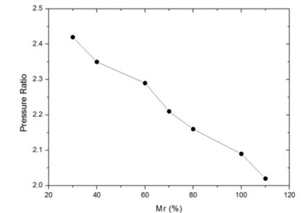
Total pressure ratio of impeller under the different reduced mass flow conditions:
