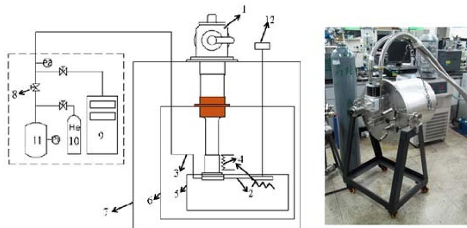
1: G-M cryocooler; 2: pre-cooling system; 3: charge tube; 4: heater; 5: 4K thermal shield; 6: first thermal shield; 7: vacuum vessel; 8: valve; 9: vacuum pump; 10: gas cylinder; 11: buffer tank;
