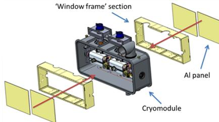
Thermal shield assembly sequence
