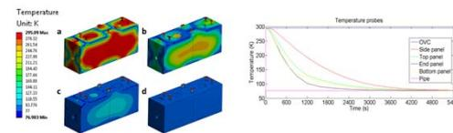
Temperature profile during fast cooldown at a) 72 s, b) 588 s, c) 2306 s and d) 5400 s (~steady state condition)
