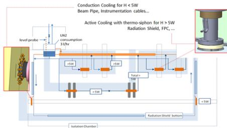
Schematic for cooling to 80K with LN2
