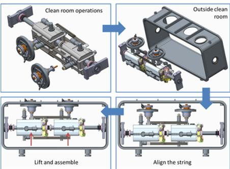
Cryomodule assembly sequence
