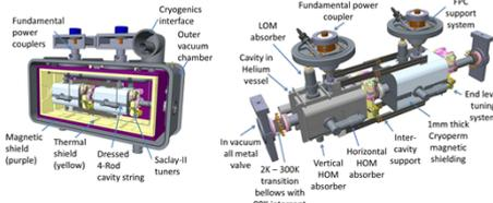
Side loaded cryomodule and the dressed cavity string
