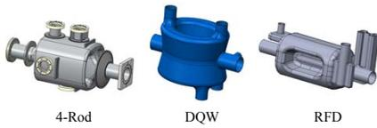
Several cryomodule designs corresponding to three different cavity designs, 4-Rod, Double Quarter Wave (DQW) and RF Dipole (RFD), were considered
