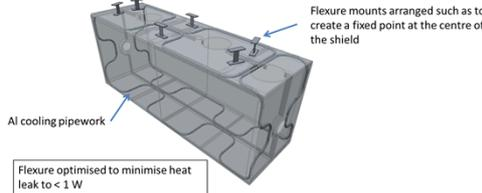
Thermal shield (including flexure mounts)
