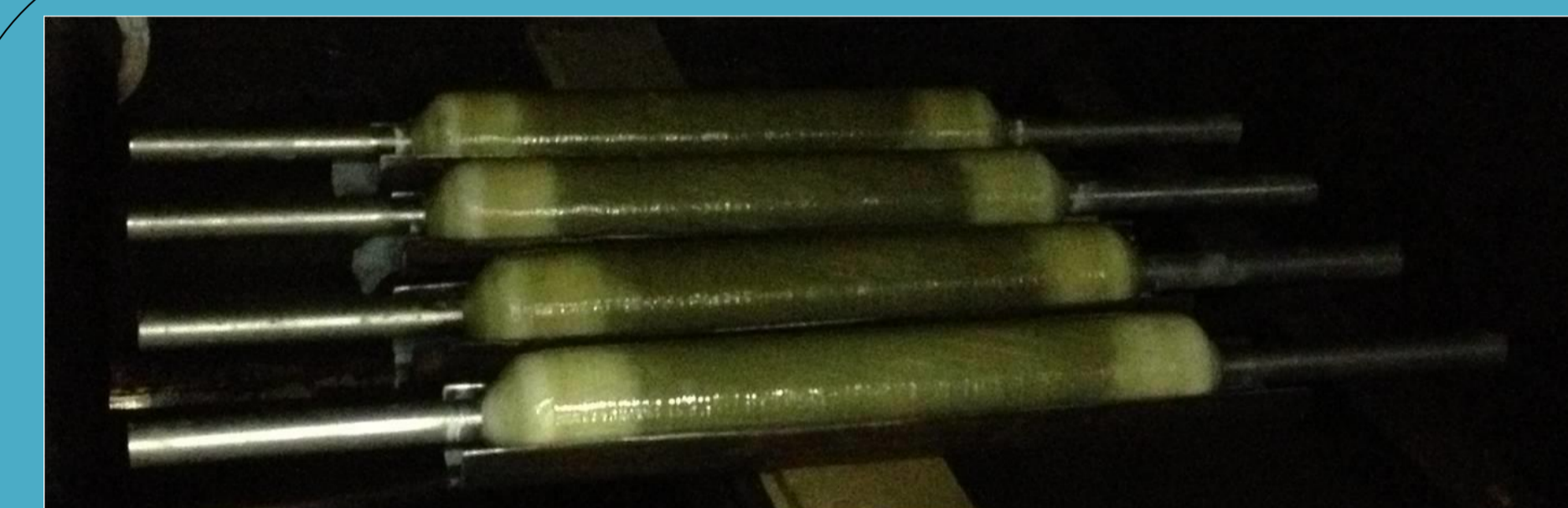
30kV HV IBs in the oven
