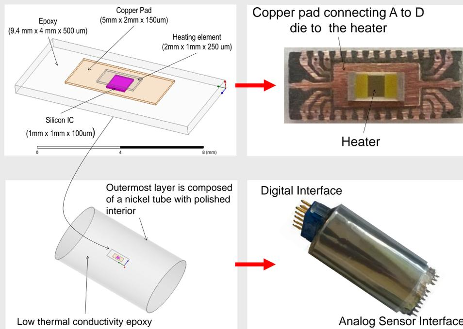
The set of pictures on the left illustrates the thermal package assembly. The A to D converter ASIC die is located on the other side of the copper pad. The A to D consumes only 400uW, while the heater used to maintain the A to D operating temperature consumes 40mW for the current prototype. This will be dramatically improved in the next version, when a much lower thermal conductivity insulator will be utilized for the outer layer of the package.
