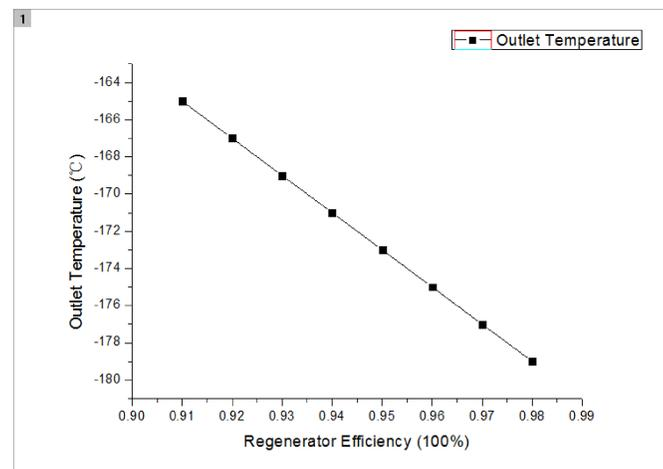
With the increase of regenerator efficiency, the outlet temperature dropped linearly. This temperature drop means higher regenerator efficiency will contribute to storing more cold energy.
