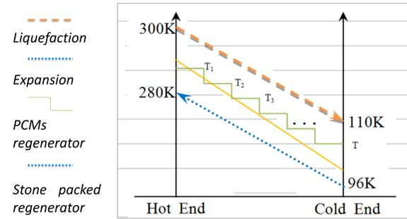
Temperature gap between two ends in stone packed regenerator is larger than that in PCMs regenerator. Therefore, regenerator with PCMs is expected to have more stable performance.
