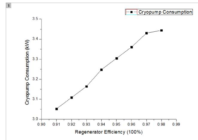
Cryopump tended to consume more electricity as regenerator efficiency increasing. This tendency means the flux in cryopump was increasing. Further, it implies the amount of liquid air stored in cryo-tank was increasing.
