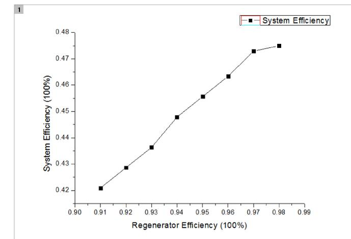
The compressor set consumption was constant in this simulation, therefore, system efficiency defined as output over consumption increased obviously with the increase of regenerator efficiency.
