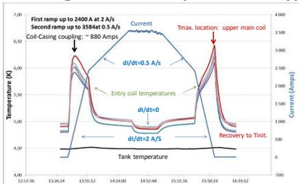
The maximum initial coil temperature is 4.97 K at the entry of lateral upper coil. The temperature at the entry of main upper coil increases up to 6.23 K, this maximum is observed during the current ramp-up for all coils, always at a current of ~ 880 Amps; This temperature limit is certainly due to the occurrence of a better thermal contact between coils and casings, caused by the mechanical coupling strength, proportional to the square of the current.
