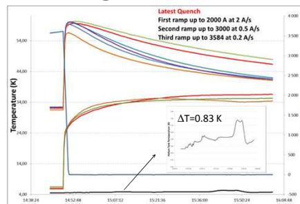
During the quench, the maximum coil temperature is 59.3 K, while the maximum casing temperature is 36.6 K. This ΔT value of about 30 K was well predicted by the simulation.
