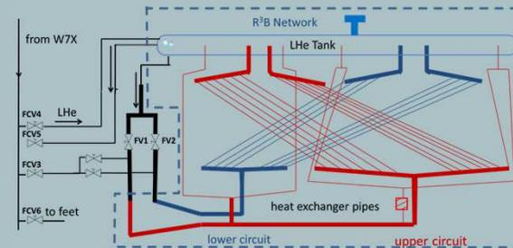
Schematic view of the cryogenic connection between “W7X” test station and R<sup>3</sup>B-Glad
