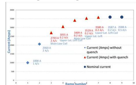
On 5 December 2013, the cold mass reaches its nominal current of 3584 Amps after five training quenches, due to mechanical adjustment movements of the coils inside their casings.
