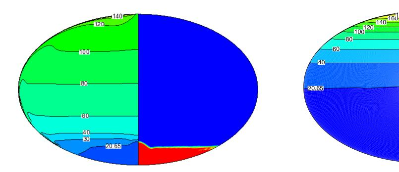
Temperature and phase field during LH2 fill process (7.5 kg/s):(a) 100 s;(b) 1000 s
