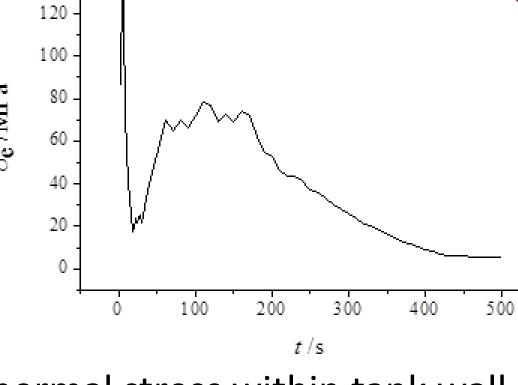
Thermal stress within tank wall during LH2 fill process (7.5 kg/s): (a) time history of the maximum value; (b) axial distribution.
