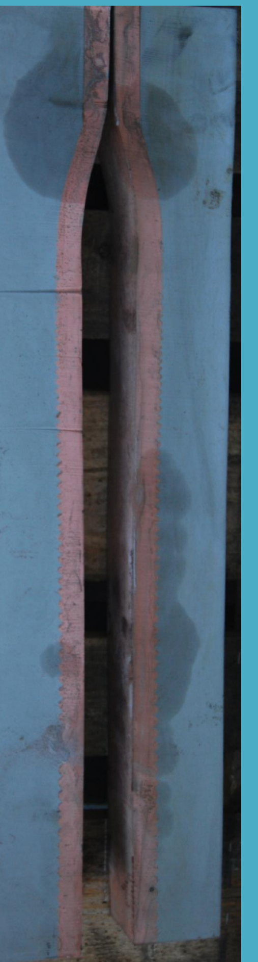
Tails for load transfer from testing machine
