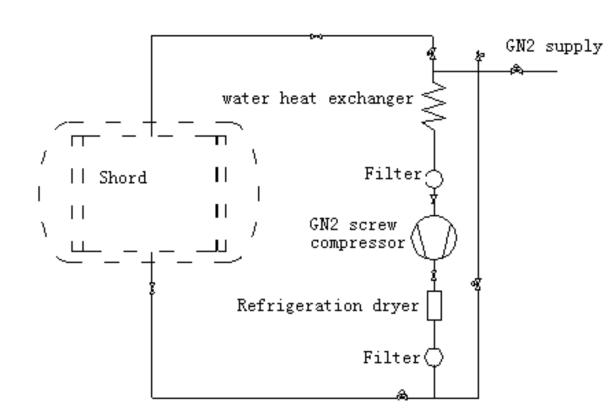
Working principle of GN2 subsystem
