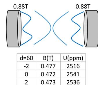
When settled face-to-face, we obtained 2,516 ppm of 0.477 T at 60 mm gap
