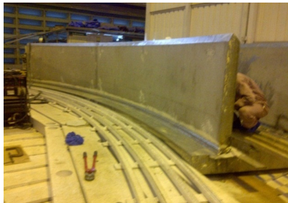
Cryostat pedestal ring- bottom plate (180 mm) & side plates (120 & 80 mm) are being welded together
