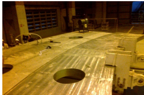
Cryostat pedestal ring- top plate 200 mm and skirt plate 105 mm thick welded together
