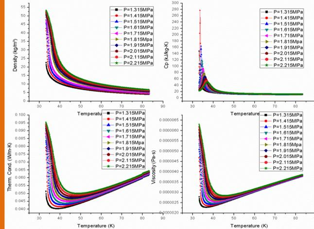
Figure 1. Density, Thermal conductivity, Specific heat and Viscosity at varying temperature and pressure.
