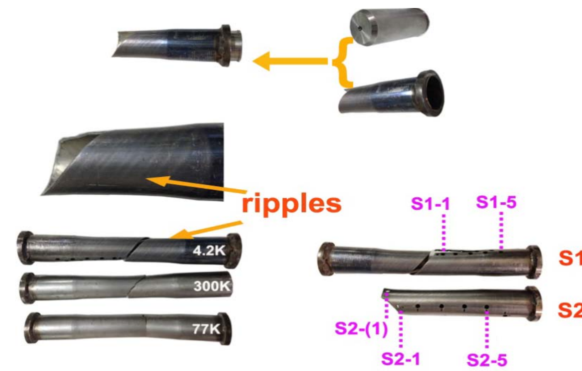
Fig. 1. The optical images of the fractured full-size tubes at 4.2K, 77K and 300K.
