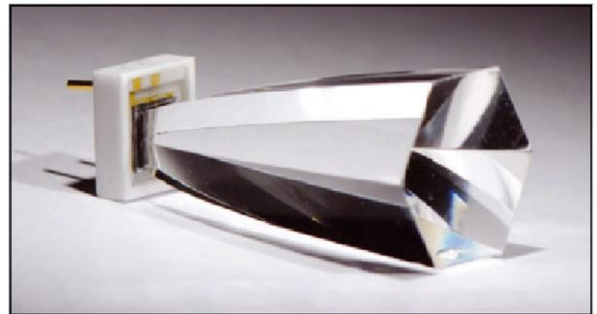
A single G-APD, only 2.8 \times 2.8 \text{ mm}^2 , glued to its light concentrator.
