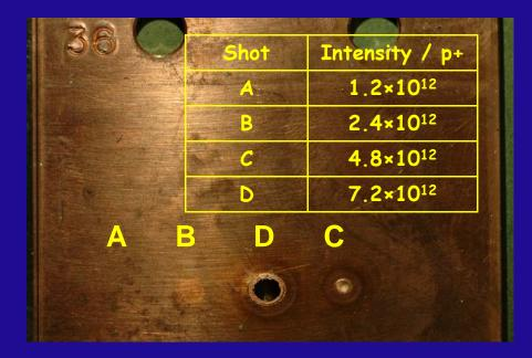
Based on those results the MPWG has adopted for the LHC a limit for safe beams with nominal emittance @ <u>450 GeV</u> of:
