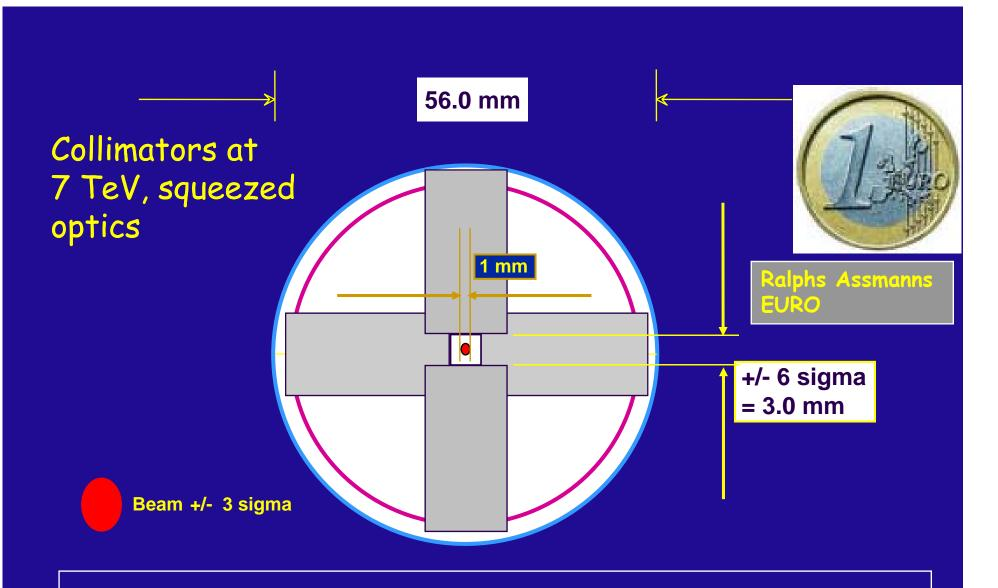
Example: Setting of collimators at 7 TeV - with luminosity optics Very tight settings  $\rightarrow$  orbit feedback !!
