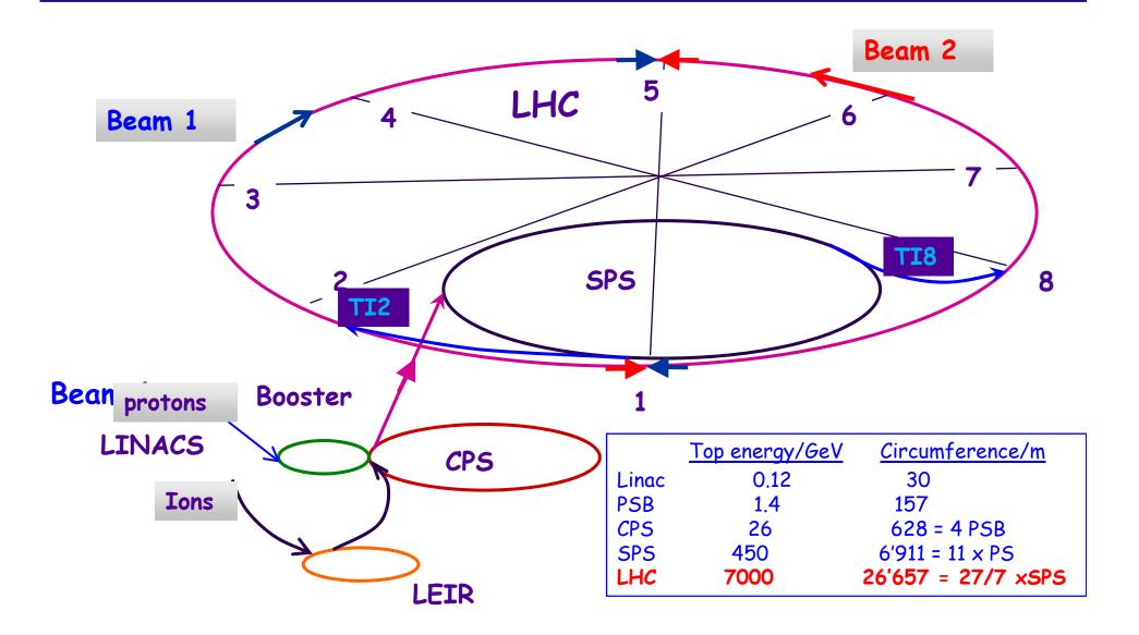
Note the energy gain/machine of 10 to 20 - and not more ! The gain is typical for the useful range of magnets !!!
