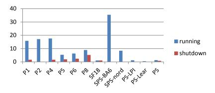
**Energy dissipation on cooling towers [MW]**
