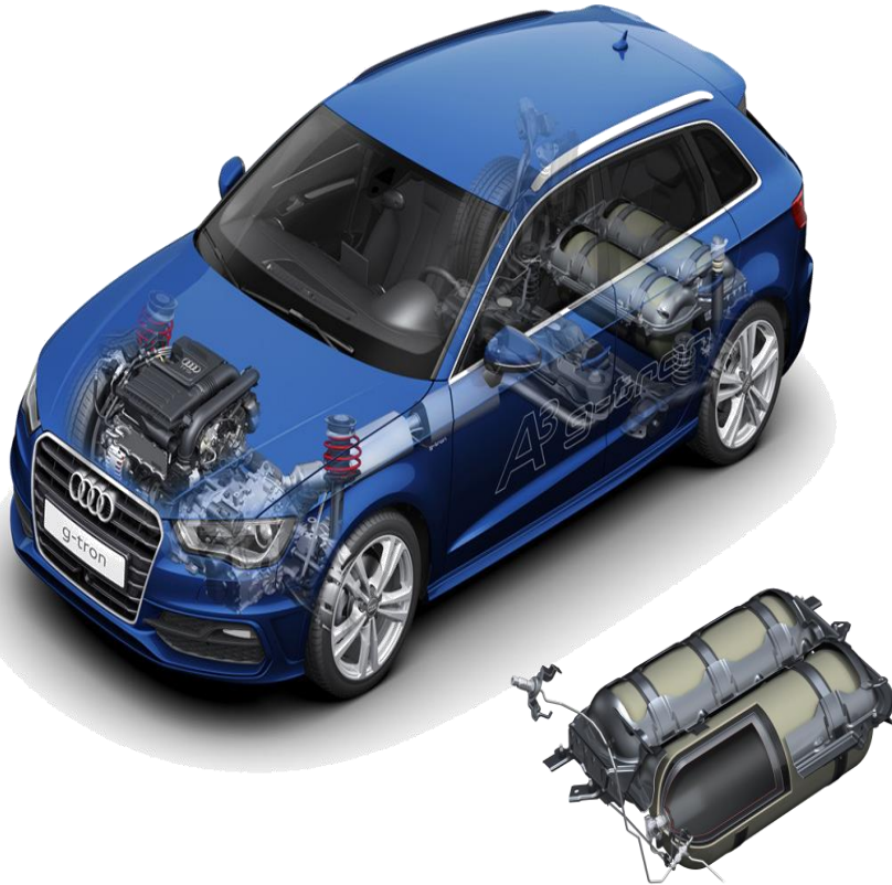
Audi A3 g-tron: natural gas tanks
