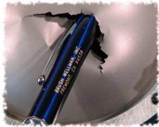
Intentionally broken 50 \mu m thick Be speaker dome
