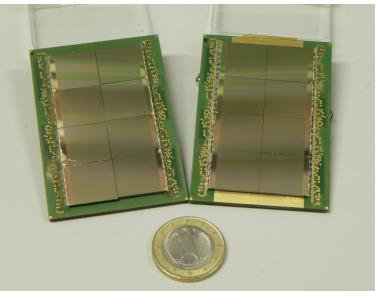
Used as readout anode plane in gaseous detectors
