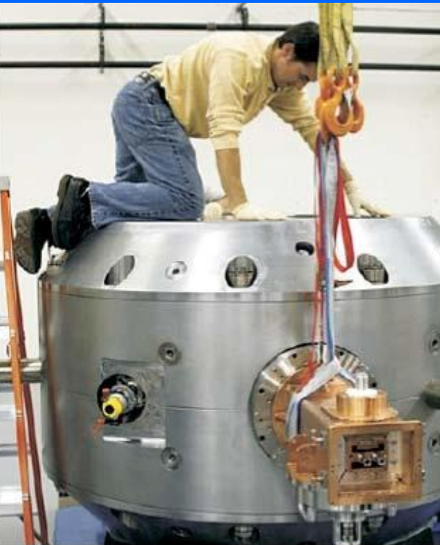
9 tesla superconducting synchrocyclotron
