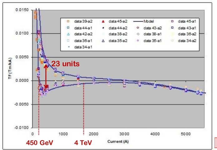
Measurement of the transfer function for MQM (similar for MQY)
