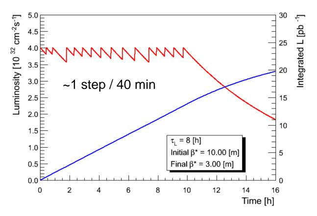
□ 25 ns beam with ~3.5  $\mu$ m emittance and 10<sup>11</sup> p/b leveled to 4x10<sup>32</sup> cm<sup>-2</sup>s<sup>-1</sup>.
