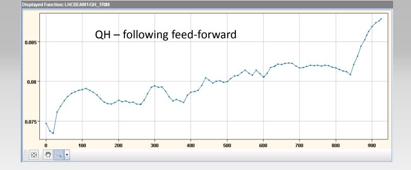
Tune correction in squeeze – corrections anywhere in time – bespoke smoothing
