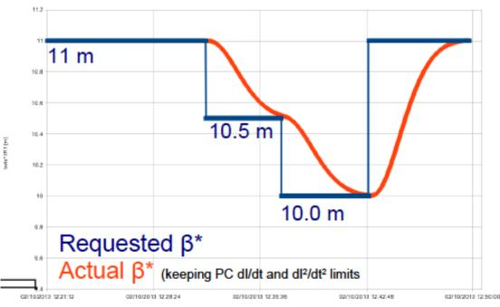
N.B. naked squeeze in IR1 only with no prior orbit, Q/Q' corrections included. 2<sup>nd</sup>-order feed-down effects on tune and orbit clearly observed. Beam lifetime OK throughout test → to be further studied/explored for after LS-1
