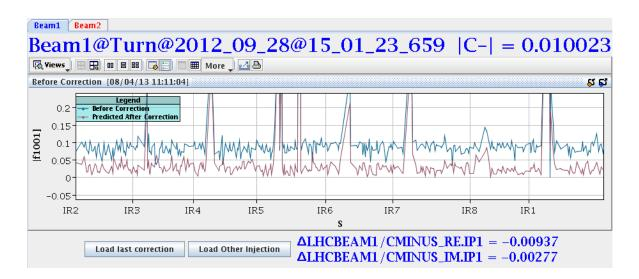
Semi-automatic Coupling correction at injection
