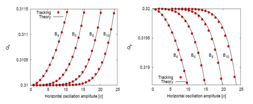
$\rightarrow$  Built a simple tracking code allowing to study driven oscillation in the presence of arbitrary non-linear field components (behavior also checked with MADX, much slower)
