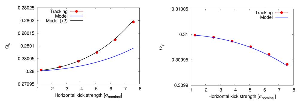
$\rightarrow$  MADX model constructed using a thin lattice with magnetic field errors from WISE of order from (B<sub>3</sub>, A<sub>3</sub>) up to (B<sub>15</sub>, A<sub>15</sub>). Includes second order effects. Example of flat top optics in this case
