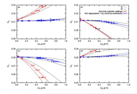
$\rightarrow$  Example of amplitude detuning measurement at the LHC
