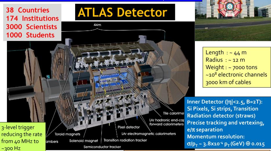
EM calorimeter: Pb-LAr Accordion e/ $\gamma$  trigger, identification and measurement E-resolution:  $\sigma/E \sim 10\%/\sqrt{E}$  HAD calorimetry ( $|\eta|<_5$ ): segmentation, hermeticity Fe/scintillator Tiles (central), Cu/W-LAr (fwd) Trigger and measurement of jets and missing E<sub>T</sub> E-resolution:  $\sigma/E \sim 50\%/\sqrt{E \oplus 0.03}$
